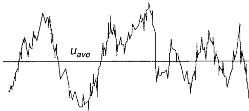
Figure 5.5-46. Velocity fluctuations at one point in the tank.
